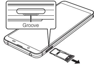
**2 Put the nano SIM Card to the nano SIM Card/microSD memory card tray with the IC (metal) side turned down.**
