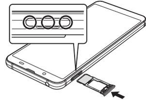
**Attaching or removing the nano SIM Card/microSD memory card tray**
