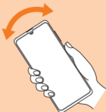
**3** Swing the product about 20 times against a dry, clean cloth etc. to wipe off water remaining in the tray eject hole, mouthpiece/microphone (upper/lower) holes, receiver, speaker, keys, headset connection terminal, external connection terminal.
