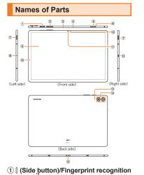
sènsor (2) Volume button (3) Microphone (upper)<sup>\*2</sup> (4) Vent hole<sup>\*2</sup> (5) SIM card/microSD memory card tray 6 Tray eject hole (7) Speaker<sup>\*2</sup> (8) Microphone (left)\*2 (9) Display (touch panel)\*3 10 Light sensor 1 Front camera\*3 (i) USB Type-C<sup>™</sup> connection terminal (external connection terminal) (13) Microphone (back)\* (14) Rear camera\* (15) Pogo pin 3
