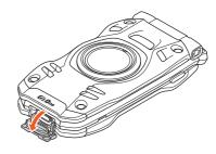
Insert the USB Type-C plug of Type-C Common AC Adapter 01 (sold separately) straight into the external connection terminal
