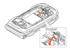
6 Install the battery pack and back cover
