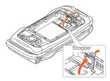
4 Slide the SIM card in the direction shown below with the terminal (metal) part downwards until it clicks
