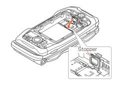
6 Install the battery pack and back cover
