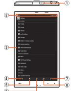
① (Power key): Hold it down to turn the power on. Hold it down while the power is turned on  $\rightarrow$  [Power off]  $\rightarrow$  [OK] to turn it off.
