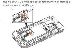
Slide the au Nano IC Card (LTE) slot cover with the pad of
