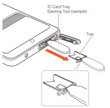
Put the au IC card on the tray with the position of the card's notch adjusted, then insert the tray straight into the au IC card slot (lower side)
