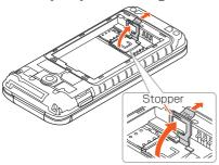
4 Push the au IC card (SIM card) until it clicks (1), and then slide the card to remove (2)
