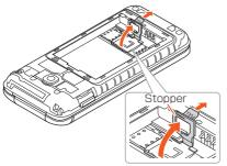
4 Slide the au IC card (SIM card) in the direction shown below with the terminal (metal) part downwards until it clicks
