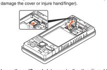
Slide the au IC card in the direction shown to remove Lower the au IC card slot cover in direction ①, and then slide in direction ② with the pad of your finger until it clicks locked
